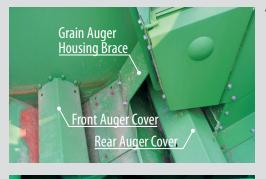
Remove front auger cover, as shown in the picture at the immediate left. It may be necessary to remove the drive shaft housing, as shown in the picture at the lower left. Next, remove the clean grain auger housing brace and then the rear auger cover. *Do not remove the augers*.
