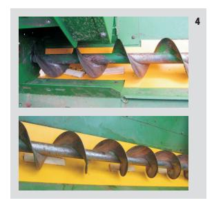
Wedge the liner down using the wooden wedges supplied, as shown in the pictures at left, being sure the liner is centered under the auger along the entire length.
