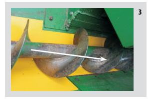
Starting with the rear (upper) auger, insert the poly liner under the auger. Slide the liner to the right until it makes contact with the vertical wall of the tank.
